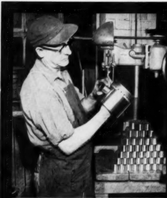
Gardner-Denver workman inserting a Johnson sleeve bushing in a compressor piston.
